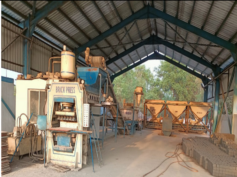
Figure 7 Ash utilization in brick manufacturing for own use
