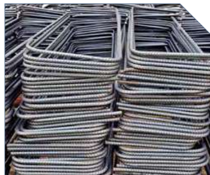
Cut and bend rebars
